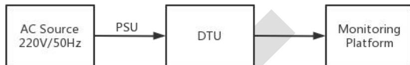
Figure 1 RE Test configuration
